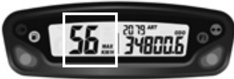
Fig 2 MAX speed function
